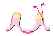
Spherical deformation in conjunction with conventional polymerization according to Prof. Dr. K. H. Körber, Kiel (Germany)
